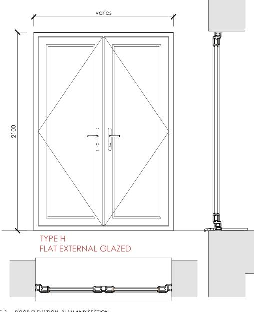
DOOR ELEVATION, PLAN AND SECTION 2 scale 1:20
