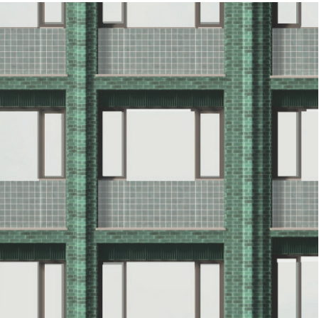
Lab Facade Bench height glazing Glazing Ratio: 40%
