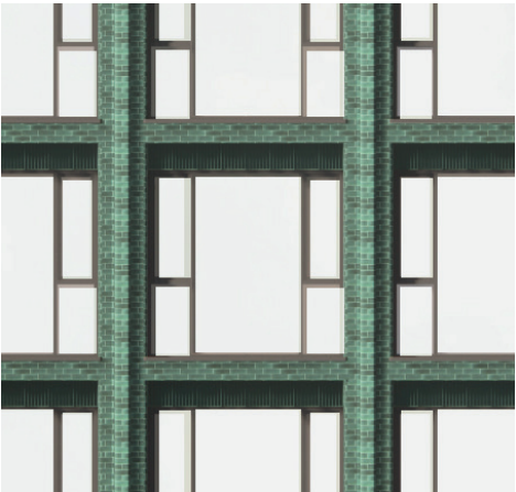
Office Facade Full height glazing Glazing Ratio: 59%
