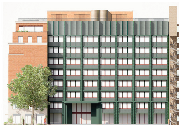
Sealed envelope Windows restored and balconies removed to allow sealed envelope
