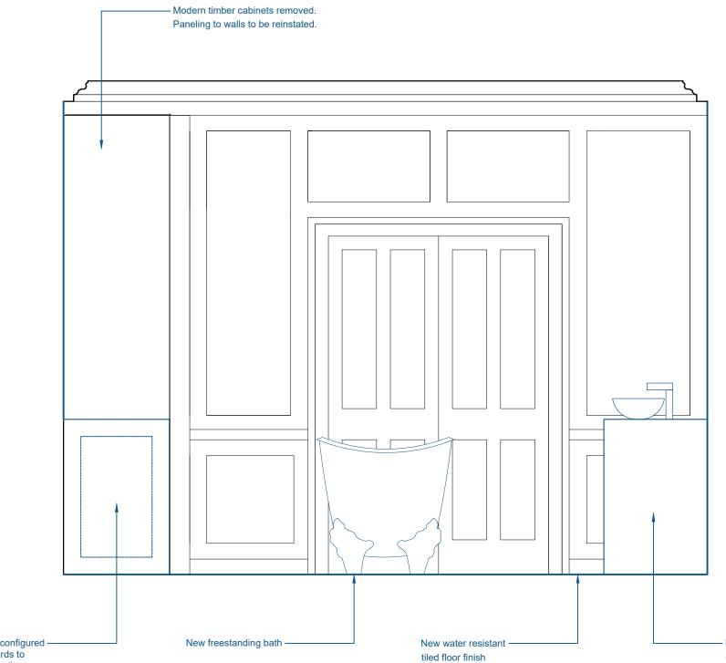
Existing MVHR system reconfigured – into new low level cupboards to services engineer's information.
