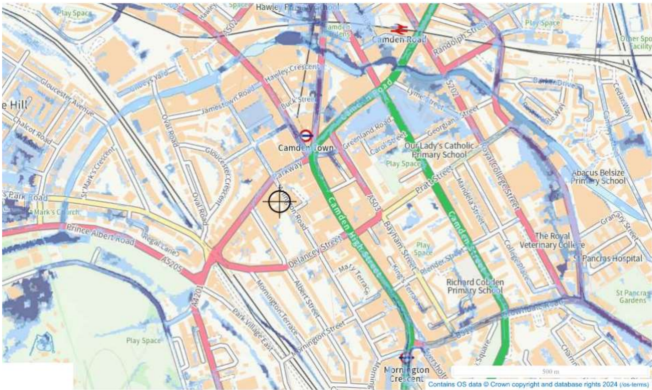
Fig 55: Flooding – Environment Agency’s Surface Water Flood Risk
