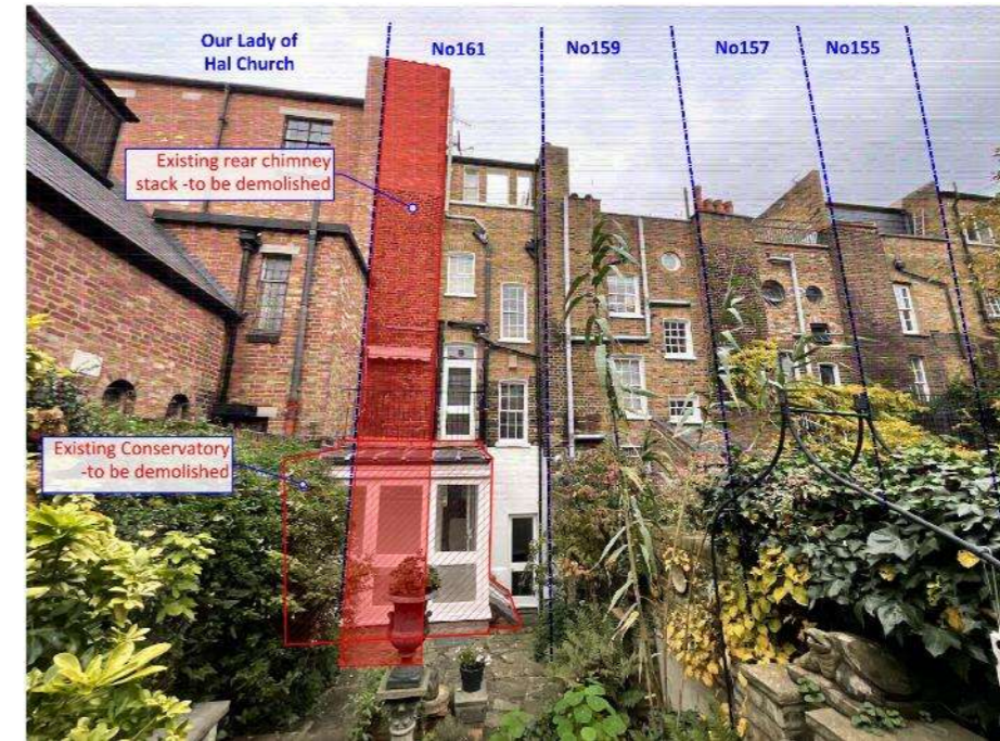
Figure 6: Rear Elevation Showing demolition
