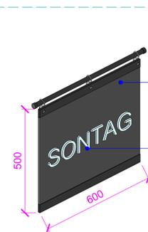
Prefabricated black power-coated metal board. RAL 9005
