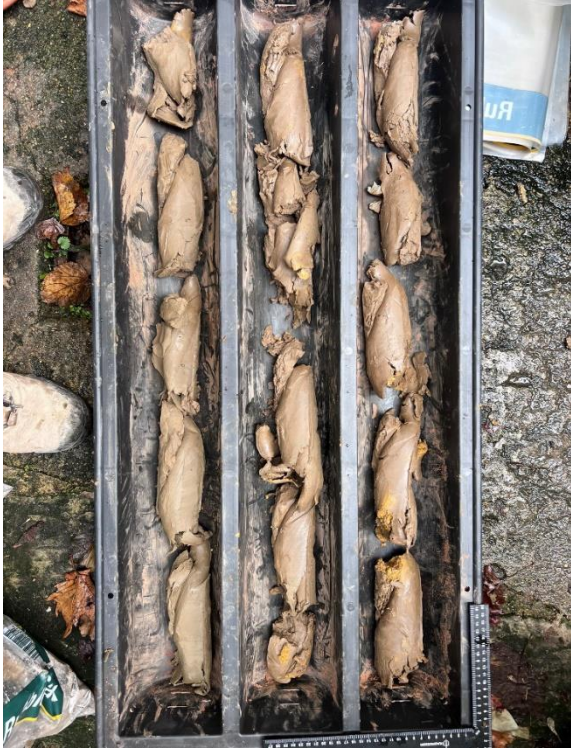
Photo 5 – BH1 Cores (1.50m – 3.00m)
