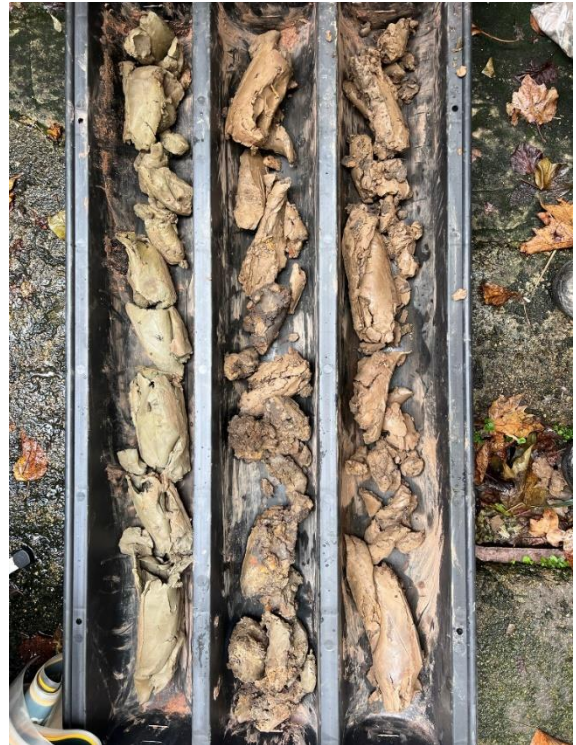
Photo 4 – BH1 Cores (0.00m – 1.50m)
