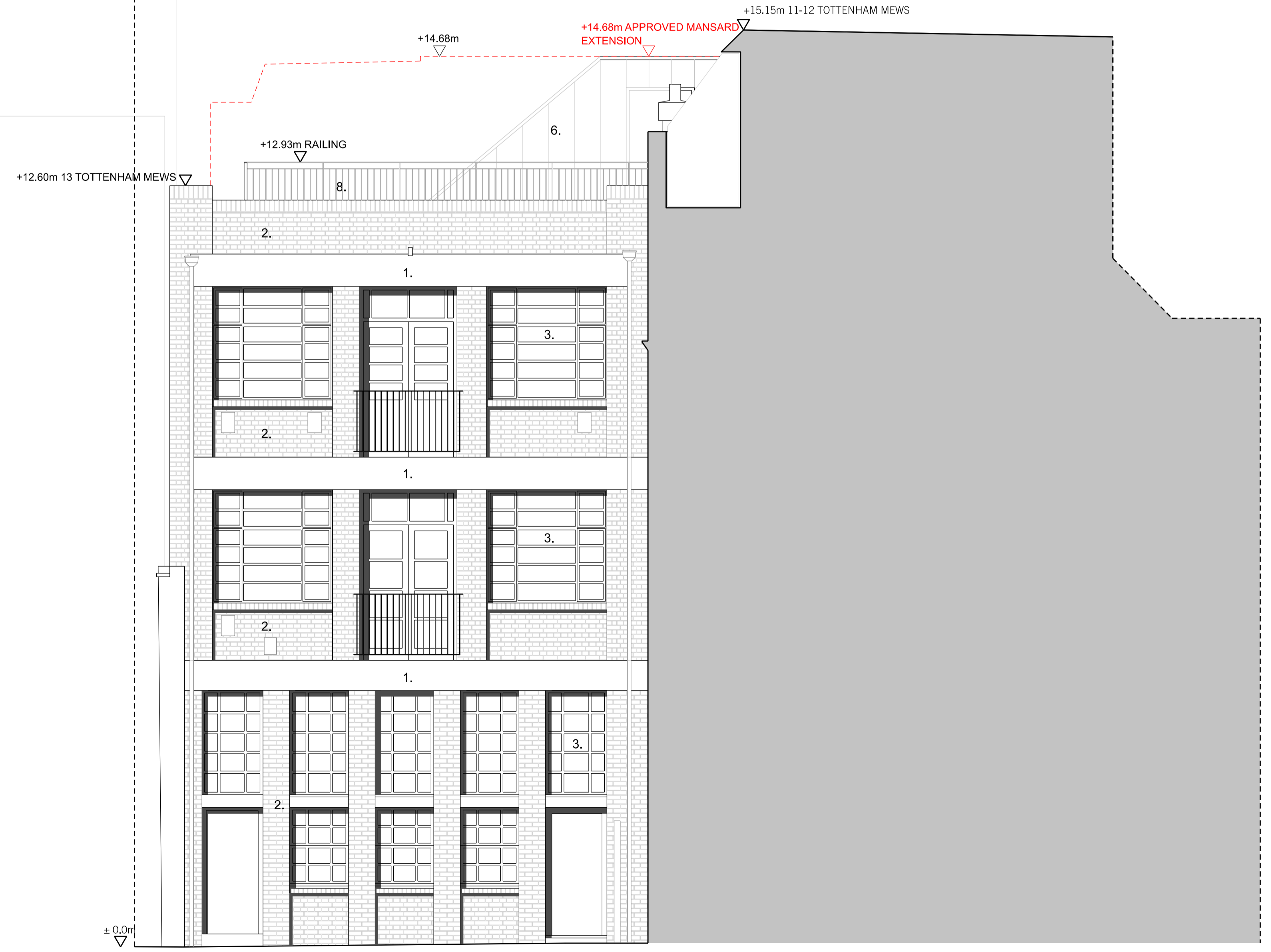
01: PROPOSED SOUTH ELEVATION SCALE 1:50
