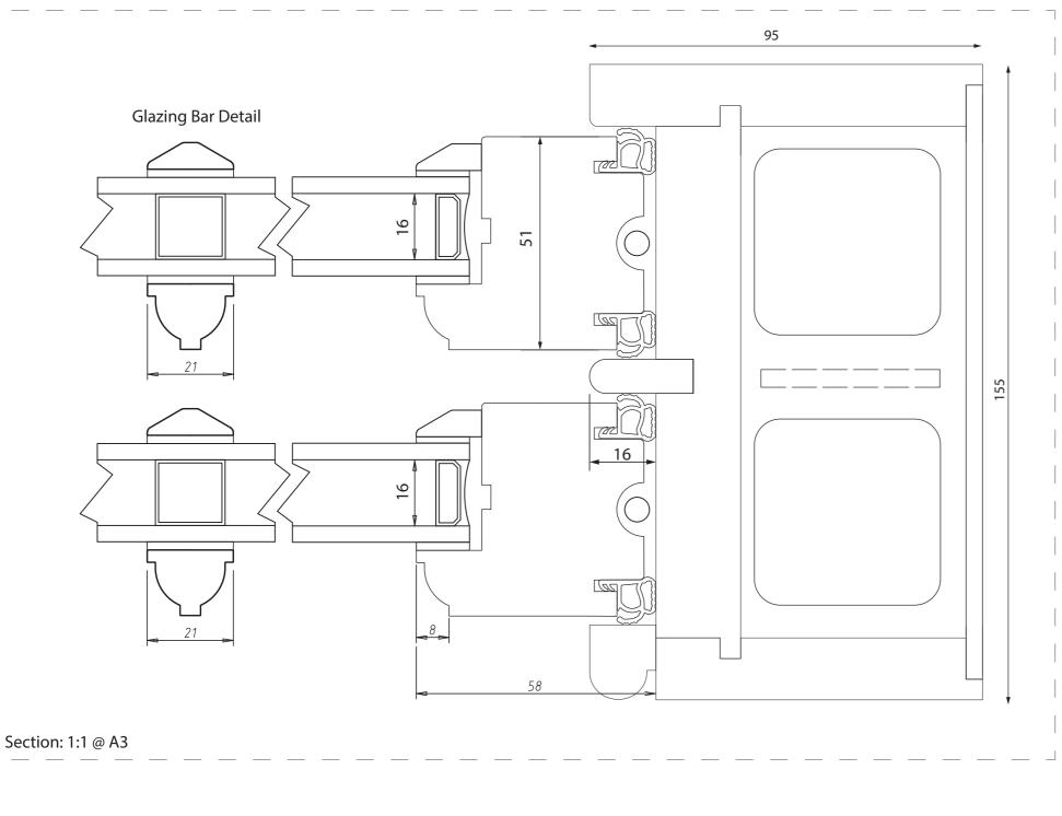
Timber: Sash window box frames and sashes are made from Accoya® wood. Our double-glazed sash windows are all hand-made using traditional mortise & tenon, glued and wedged joinery with modern techniques.
