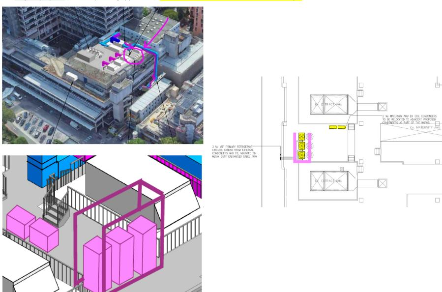
• New proposal: the Acoustic screen would be modified to show as a 'L' shape, dimensions 2.5m Height, 6.3m Length, 4.5m width.
