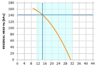
FLOW OF WATER TO HEAT EXCHANGER - Q [m3/h]
