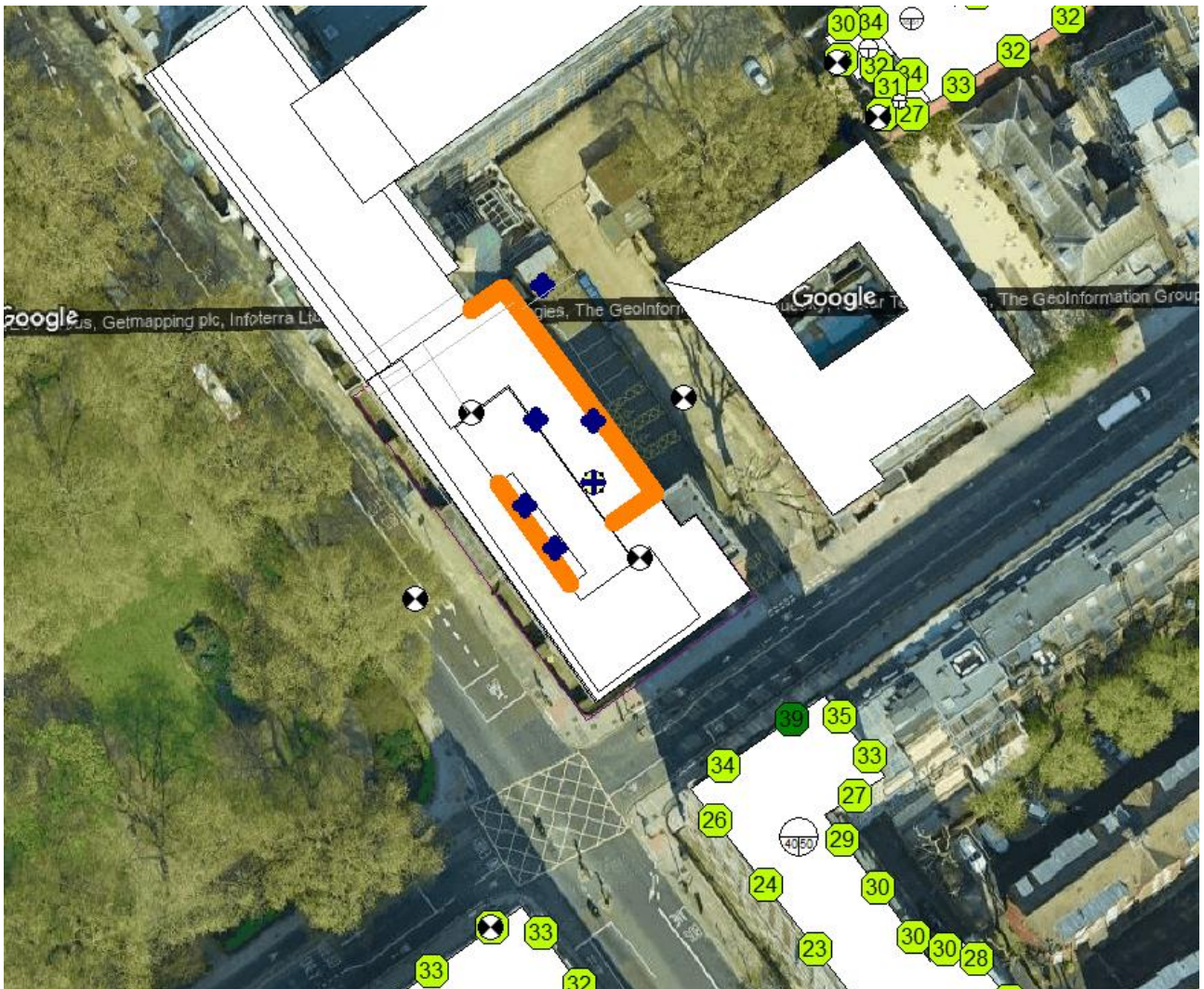
Figure 3: Screenshot of the Cadnaa noise model - Acoustic screen (Orange line) and plant location (Blue crosses).
