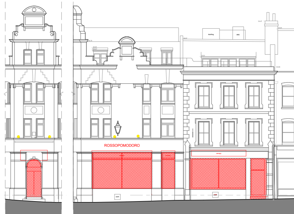
▲ Demolition Monmouth Street Elevation
