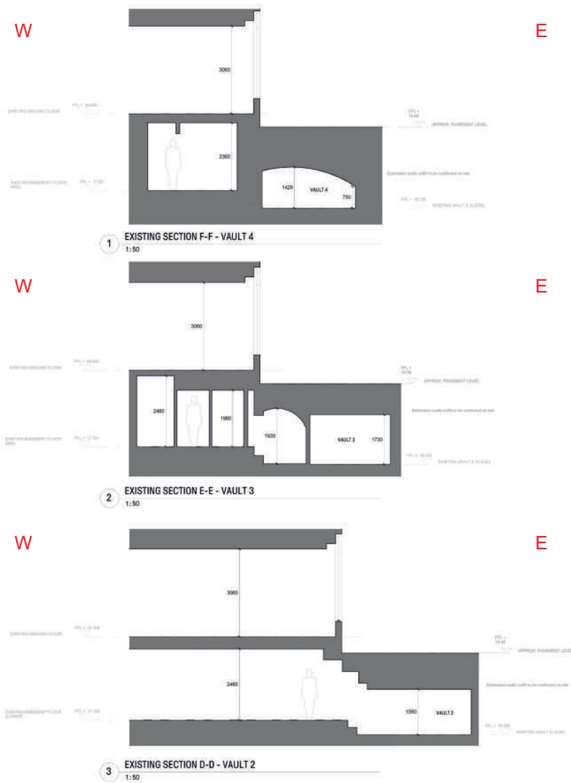
Fig 17 Existing vault sections D-D, E-E, F-F (Child Graddon Lewis, Dwg. CGL- Z1-XX-DR-A-PL1041, Rev. -, 09/02/2024)
