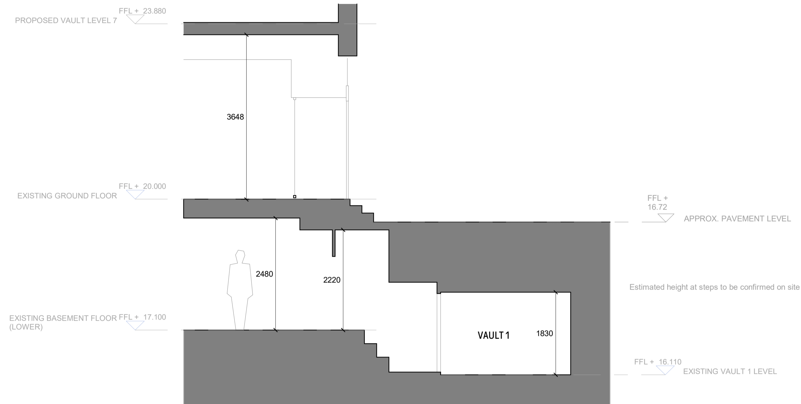
2 EXISTING SECTION C-C - VAULT 1 1:50
