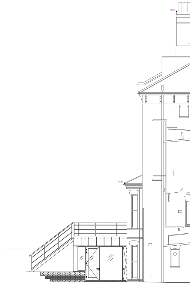
04 Proposed West Elevation / 21A Cannon Place 00_115 Scale 1:100
