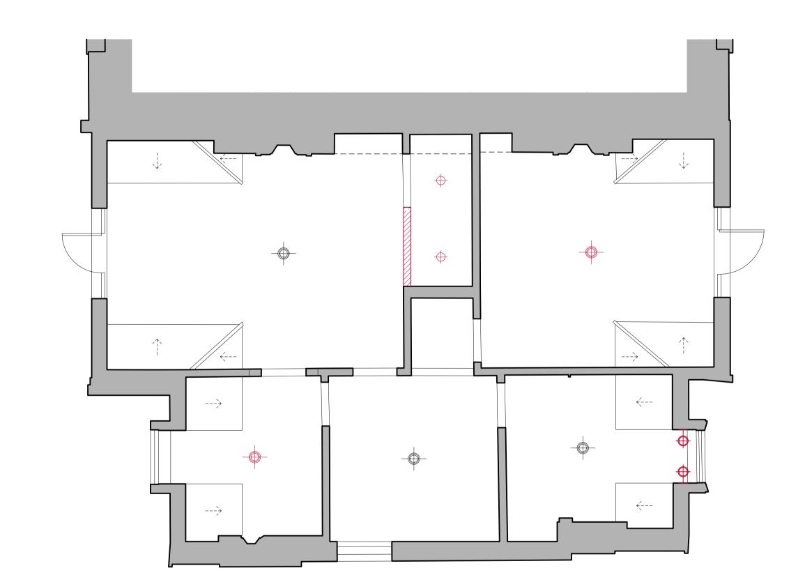
PROPOSED FIRST FLOOR RCP LIGHTING PLAN scale 1:50
