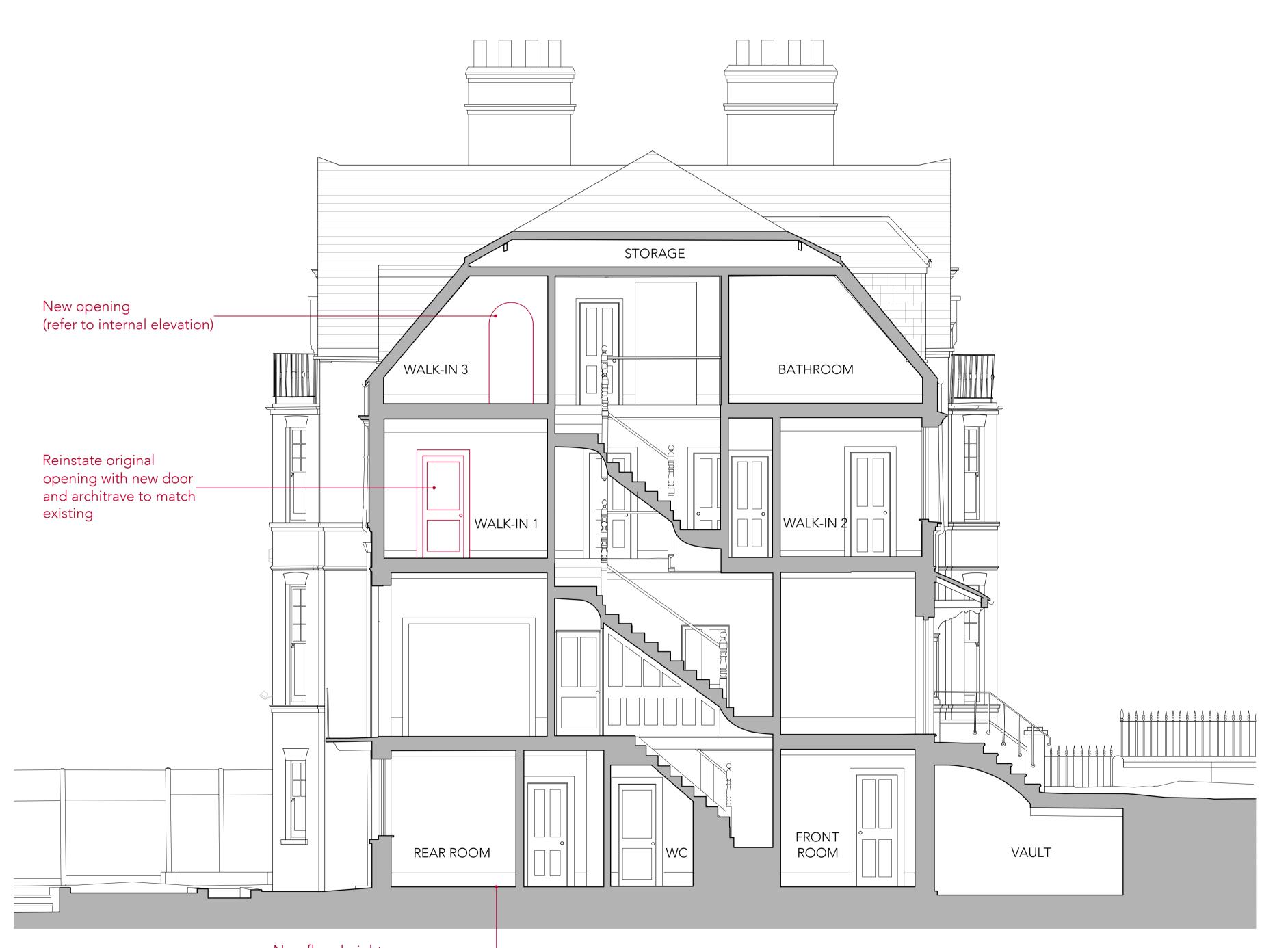
New floor height (lowered by 150mm to be levelwith existing side extension) This drawing is protected under Copyright and at no time should any portion of this drawing be reproduced or copied without the permission of the Architect.
