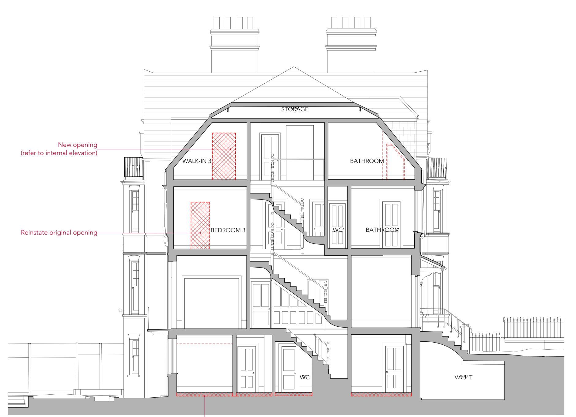
Lowering the floor height by 150mm on the entire lower ground floor to—level with the existing side extension
