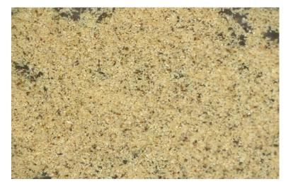
5689 Insolubles >63µm Stereomicroscope x10
