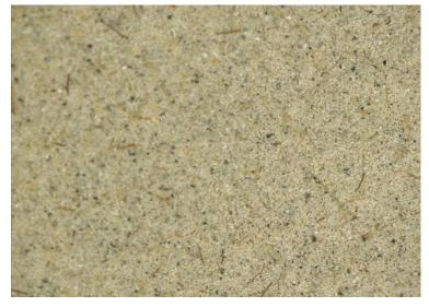
5691 Insolubles >63μm Stereomicroscope x10
