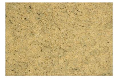
5690 Insolubles >63μm Stereomicroscope x10
