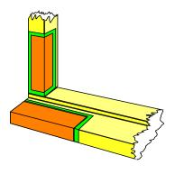
Splicing in of new timbers is easily achieved using the methods described above remembering to provide the 4mm cushion of DRY FLEX RP all round the repair. **See repair method 3**.
