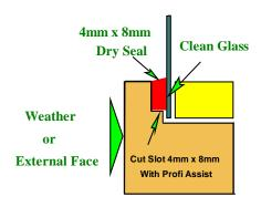
Using the PROFI ASSIST cut out the back putties to a depth of 4 - 8mm on the bottom and up to 300mm on the vertical glazing line and apply DRYSEAL elastic glazing compound in accordance with our recommendations. This will effectively seal the glazing line against moisture penetration and prevent moisture reaching the frame joints and rebates.
