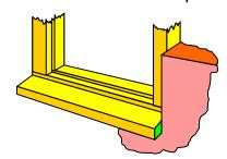
Typical example area identified in sketch: New And Existing Timbers Clean back existing timbers with Profi and to new and existing timbers apply Dry Fix and surface fill with Dry Flex RP. Sand to shape after curing.
