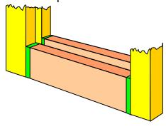
Typical example area identified in sketch: Renew decayed section complete in softwood (unprimed on meeting surfaces) to match existing section and joint to existing section at both ends with Dry Fix and Dry Flex RP ensuring a minimum 4mm joint of Dry Flex. When fully cured sand to shape ready for decoration (See Repair Method No 4).
