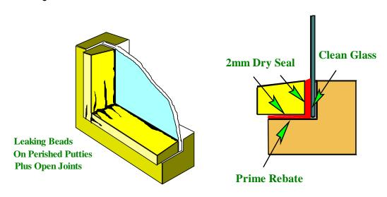
Remove bottom and side glazing beads and renew to same or revised section bedded in 2mm of DRYSEAL elastic glazing sealant. This will effectively seal the glazing line against moisture penetration and prevent moisture reaching the frame joints and rebates. See repair methods Nos 6 & 7.
