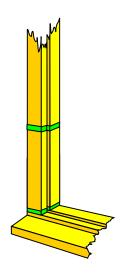
Typical example area identified in sketch: Renew decayed section complete in softwood (unprimed on meeting surfaces) to match existing section and joint to existing section at both ends with Dry Fix and Dry Flex RP ensuring a minimum 4mm joint of Dry Flex. When fully cured sand to shape ready for decoration (See Repair Method No 4).
