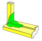
Typical example area identified in sketch: Remove decayed timber using Window Care Profi with round cutter, back to sound timber, check for excess moisture, form up as necessary with perspex slips, apply Dry Fix Wood Stabilizer and after interval apply Dry Flex RP Repair Compound to shape of timber section. When fully cured remove formers and sand sections to shape ready for decoration (See repair
