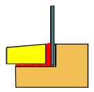
Typical example area identified in sketch: Remove all glazing beads to lower and sides of glazed openings and replace with rounded flush fitting beads (pressure treated), end grain sealed with Dry Flex SK and primed all round and bedded in Dry Seal Elastic Glazing Compound 2mm thick to both meeting surfaces (See Repair Method No 6.2 & 7)
