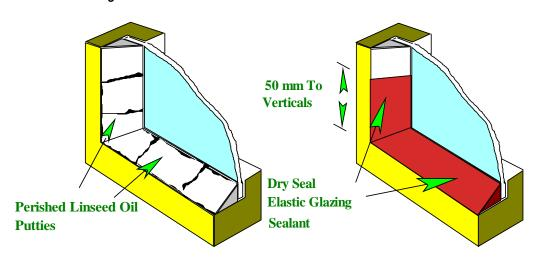
Remove bottom glazing putties including a minimum of 50mm to adjacent verticals and replace with DRY SEAL elastic glazing sealant. This will effectively seal the glazing line from moisture penetration and prevent moisture reaching the frame joints and rebates. See repair methods 6 & 7.
