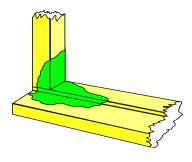
Remove decayed areas back to sound timber using the PROFI with round cutter. Check for moisture content using the WOOD CONDITION METER, apply DRY FIX, allow for penetration and fill with DRY FLEX RP. After curing, sand to shape and apply paint finish. This will give a permanent repair to the areas affected by wood decay, it will be stronger than the original timber and is flexible enough to allow movement without loss of strength or adhesion. See repair method 2.
