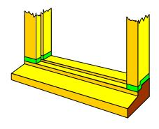
Typical example area identified in sketch: Renew decayed cill complete in hardwood/ softwood (unprimed on meeting surfaces) to match existing section and joint to existing frame and mullions with Dry Fix and Dry Flex RP ensuring a minimum 4mm joint of Dry Flex. When fully cured sand to shape ready for decoration. Assume 2 joints per 900mm (See repair Method No 4).
