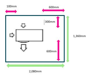
Additional maintenance access will be provided to the front elevation (discharge fan position) by either hinged or removable panels, according to the orientation of the units and the locations of accessible components. The enclosure is assumed to have no roof.
