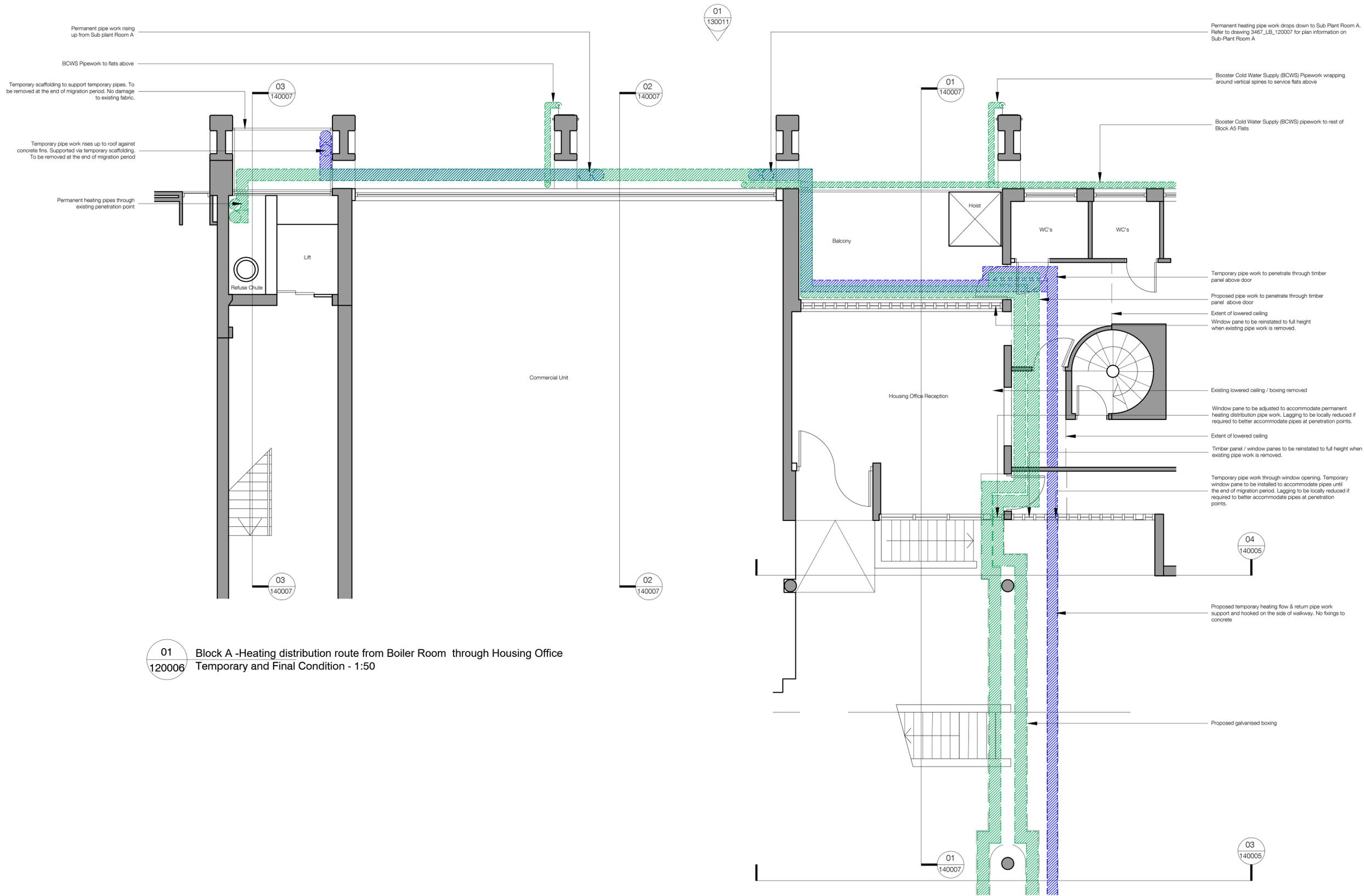
01 120006 Block A -Heating distribution route from Boiler Room through Housing Office Temporary and Final Condition - 1:50
