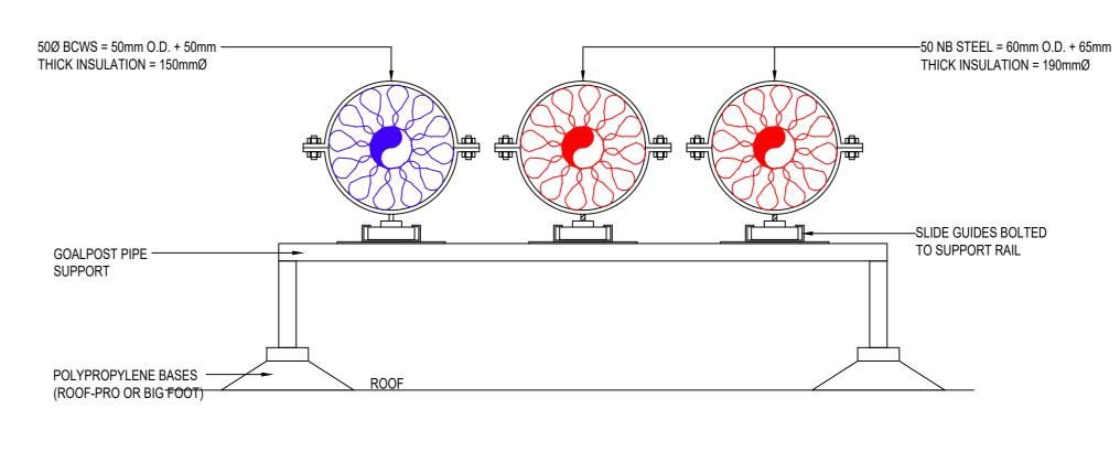
BLOCK B ROOF SUPPORTS SCALE N.T.S.
