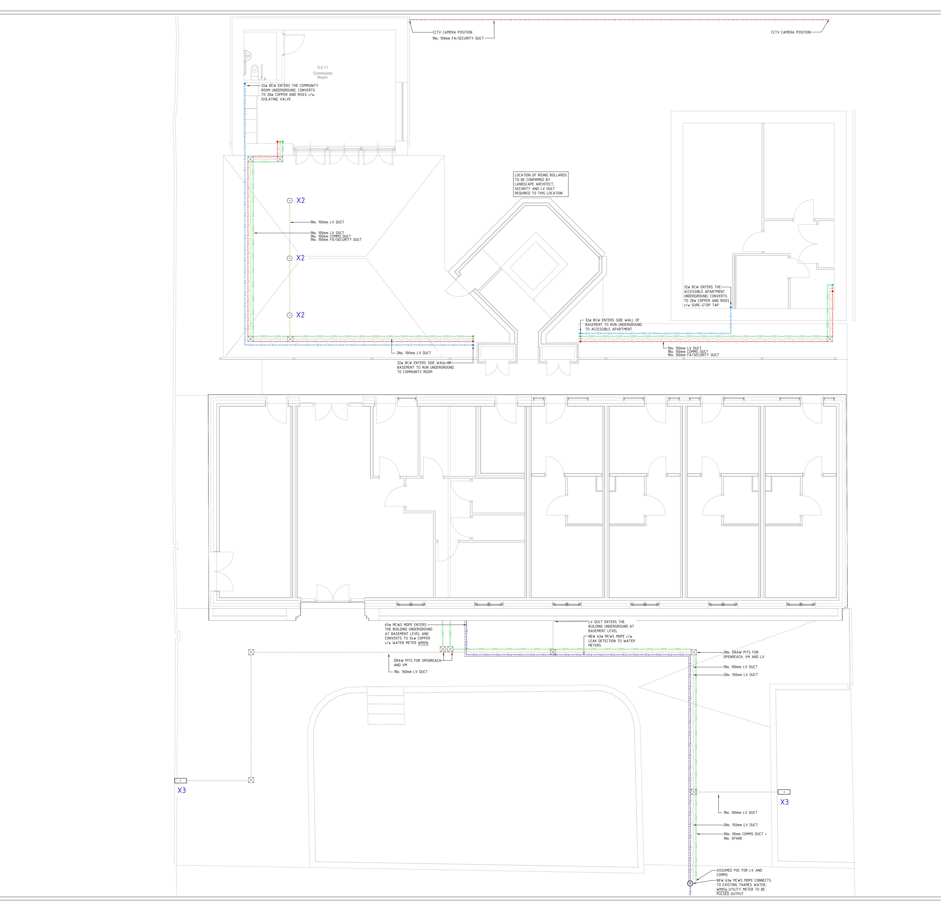
LEGEND SYMBOL DESCRIPTION ——— MCW —— MCW —— MCW ——— MAINS COLD WATER PIPE IN DUCT BOOSTED COLD WATER IN DUCT LEAK DETECTION CABLE METER DUCT ENTRY POINT THROUGH SLAB FIRE ALARM/SECURITY CABLE IN DUCT —— FA —— FA —— FA —— FA —— DATA CABLE IN DUCT
