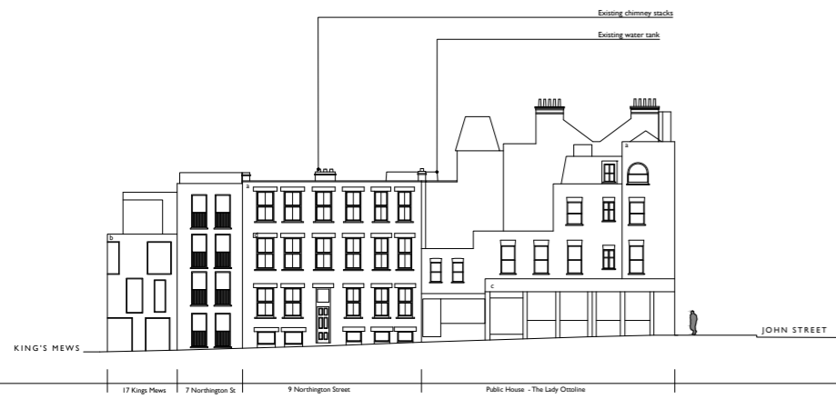
1 2018/4025/P - Existing Street Context Elevation
