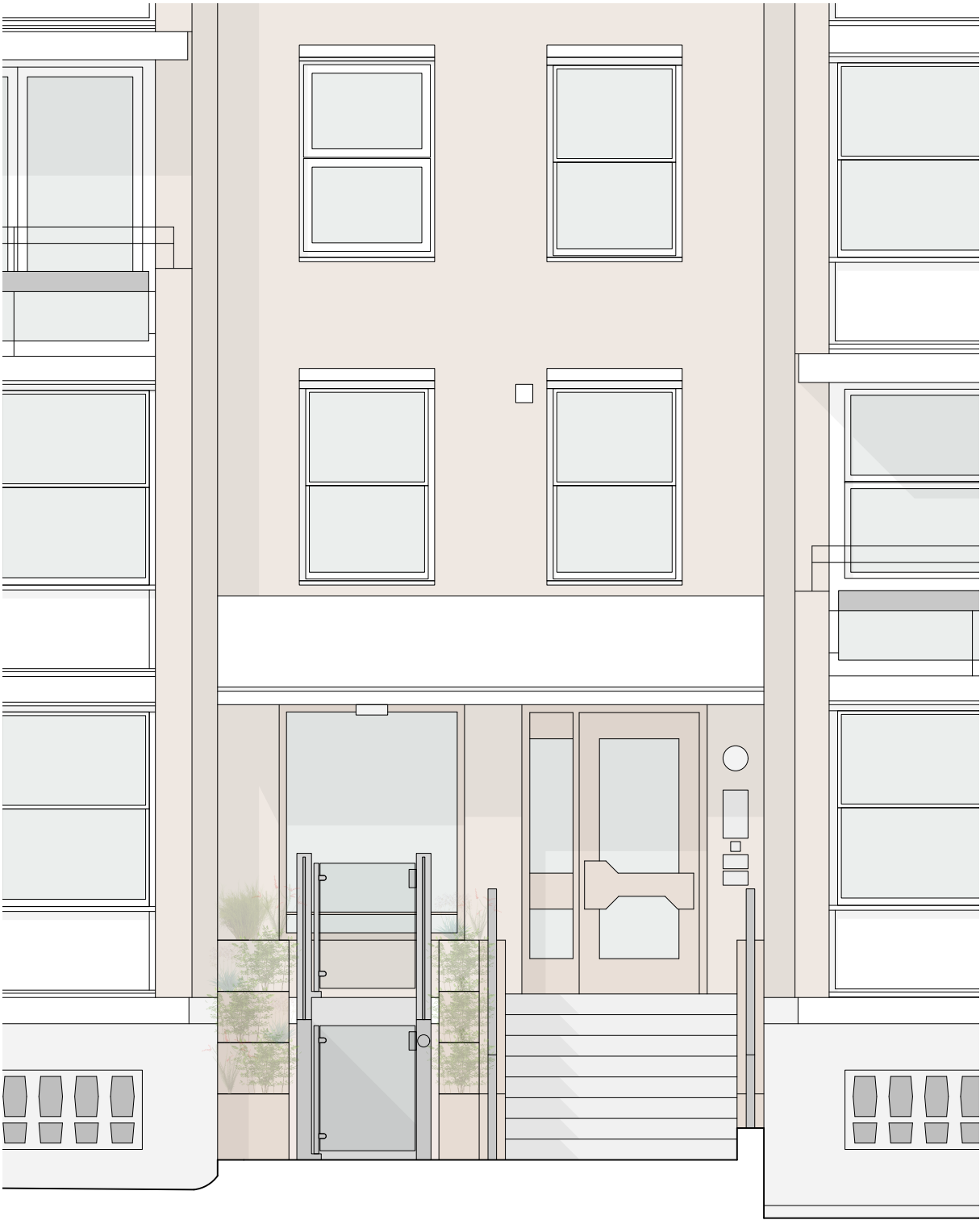
Proposed Level Access Platform Lift Elevation
