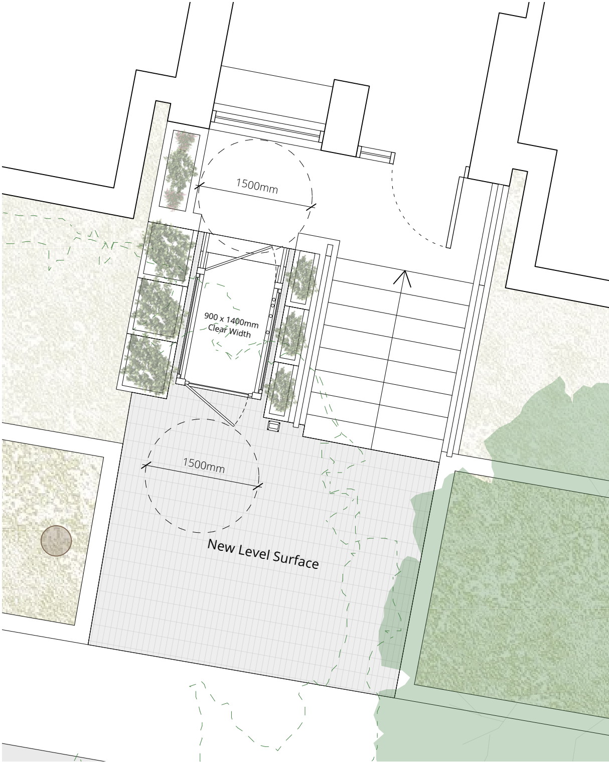
Proposed Level Access Platform Lift Plan
