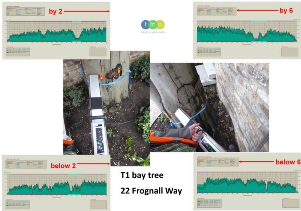
T1 bay tree RESI PD: graphs with direction and position indicated, and images of tests being undertaken.
