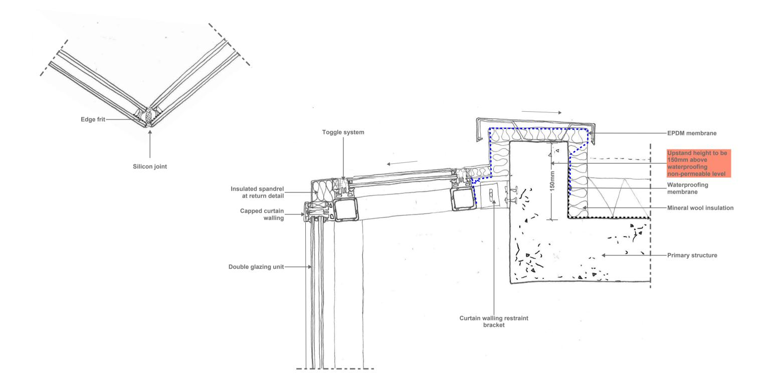
VERTICAL AND HORIZONTAL SECTION THROUGH STICK CURTAIN WALLING SCALE 1:5
