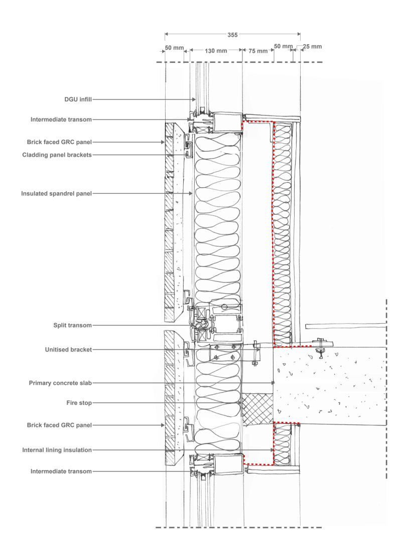
TYPICAL VERTICAL SECTION AT SLAB INTERFACE SCALE 1:5
