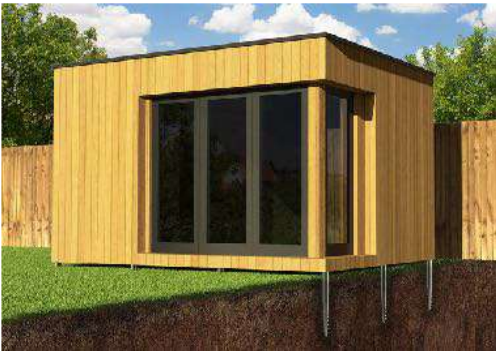
Image 02 - Example of ground screws for structural support
