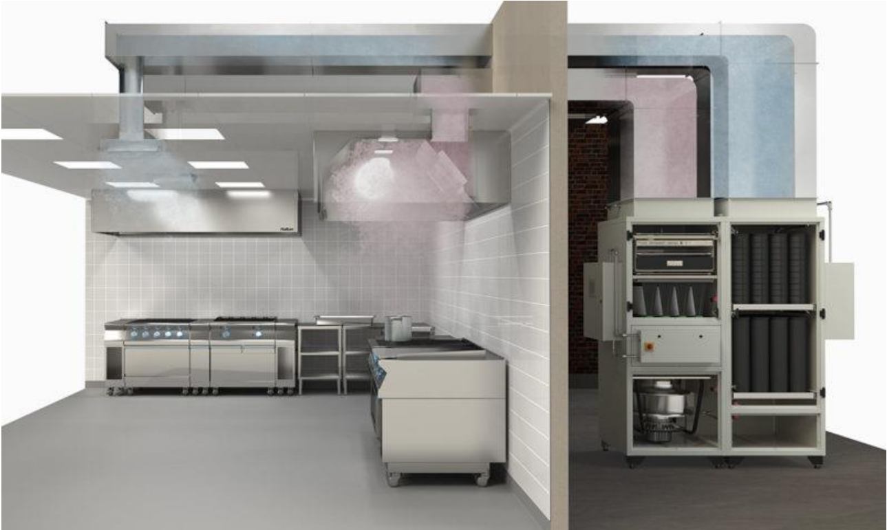
Figure 1 Typical installation of a recirculating kitchen extract unit (Image courtesy Halton)
