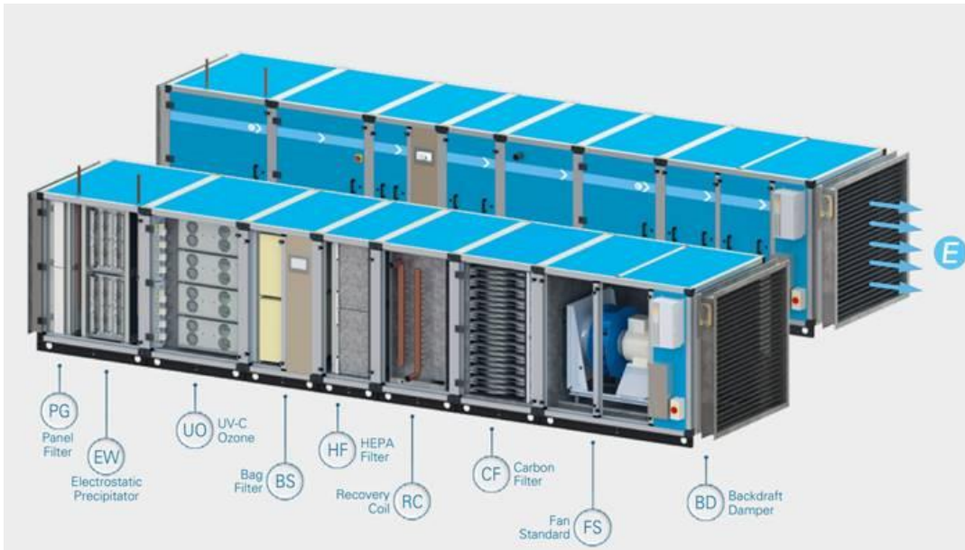
Figure 3: Typical kitchen extract air handling unit configuration
