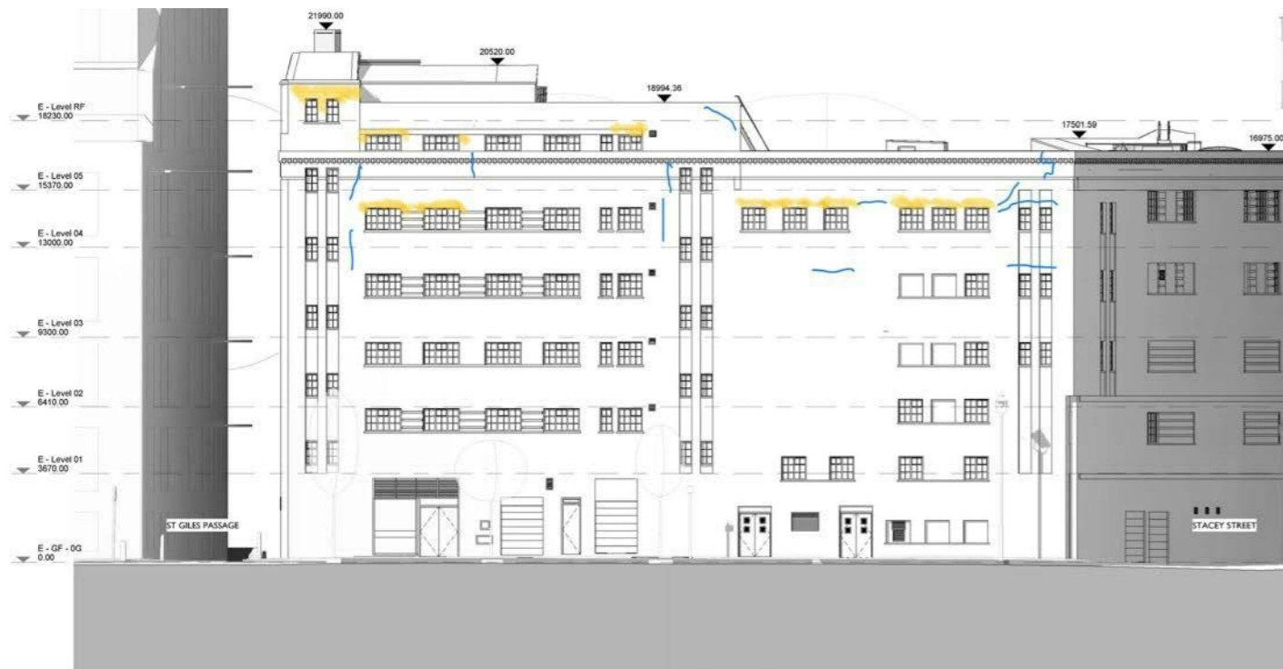
St Giles Passage elevation. Cracking visible from ground level is shown as blue lines. Areas of existing brick replacement is shown by orange shading
