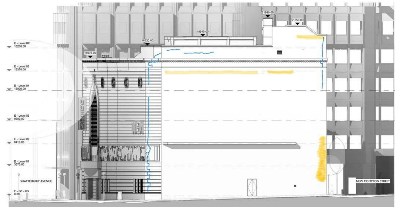
Front Elevation Cracking visible from ground level is shown as blue lines. Areas of bulging and misaligned masonry is shown by green hatching
