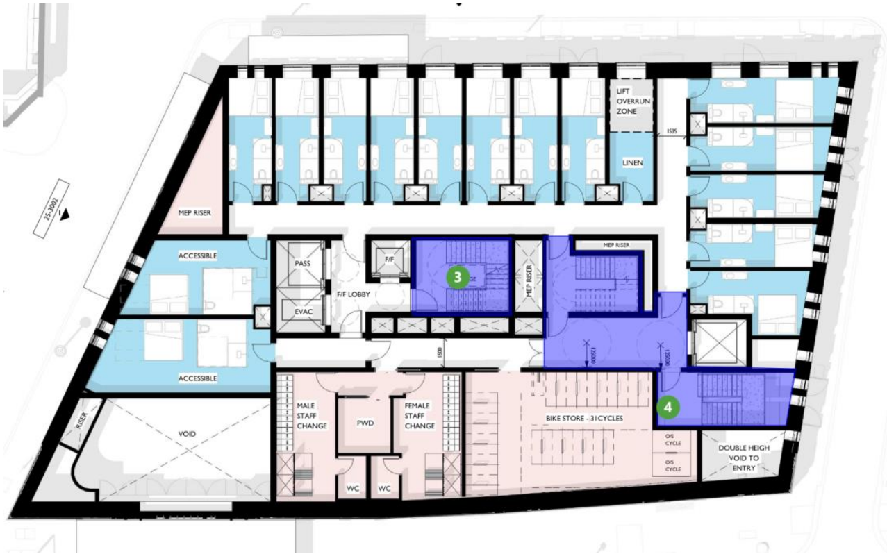
Figure 6: Level 01. Stair 4 moves from centre of the building to the South-East corner
