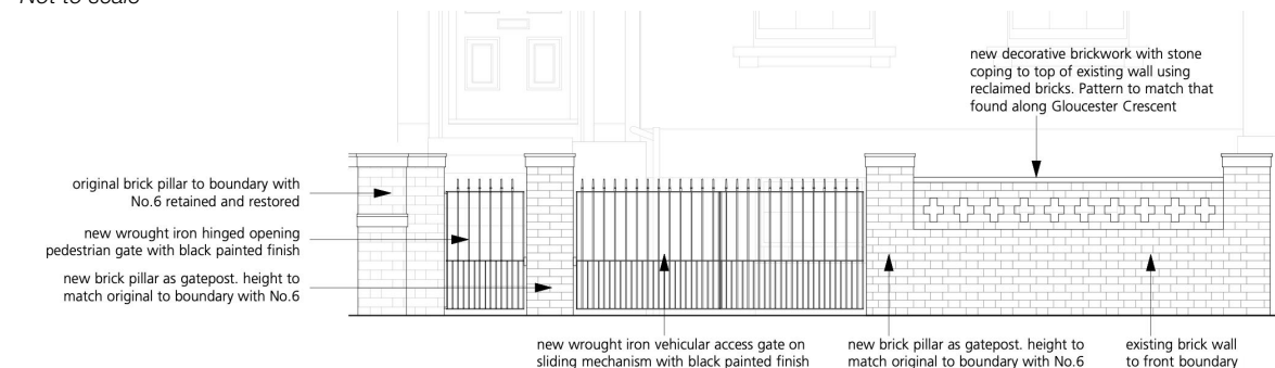
fig 2.1 - Extract of front elevation drawing submitted by others for granted application 2014/6893/L. Not to scale
