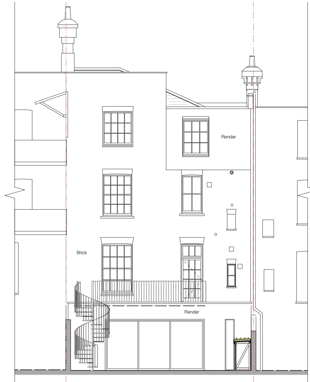
fig 4.2 - Proposed rear elevation with spiral staircase up to roof terrace and new access door at ground floor level (scale 1:100)
