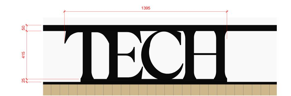
HALO ILLUMINATED SIGNAGE LED ILLUMINATION AT 4000K BEHIND OPAL ACRYLIC LETTER BACKINGS WITH BLACK LETTER FACES AND RETURNS. MOUNTED TO I BEAM DETAIL AS SHOWN ON ELEVATION DETAIL DRAWING. TOP RUNNER BAR IS NOT HALO ILLUMINATED
