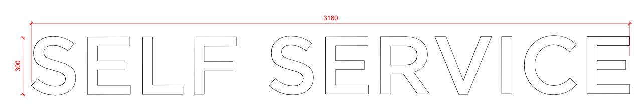
FACE ILLUMINATED SIGNAGE LED ILLUMINATION AT 4000K THROUGH OPAL ACRYLIC FACES WITH BLACK RETURNS MOUNTED INDIVIDUALLY TO BULKHEAD THROUGH FINISH.
