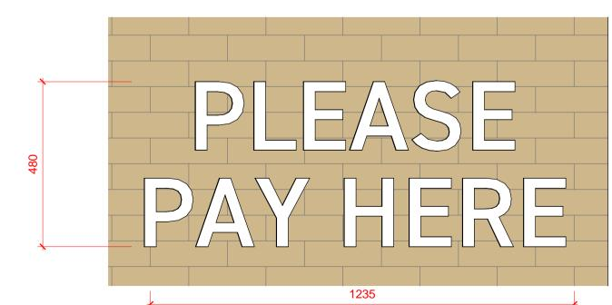
FACE ILLUMINATED SIGNAGE LED ILLUMINATION AT 4000K THROUGH OPAL ACRYLIC FACES WITH BLACK RETURNS MOUNTED INDIVIDUALLY TO BULKHEAD THROUGH FINISH.
