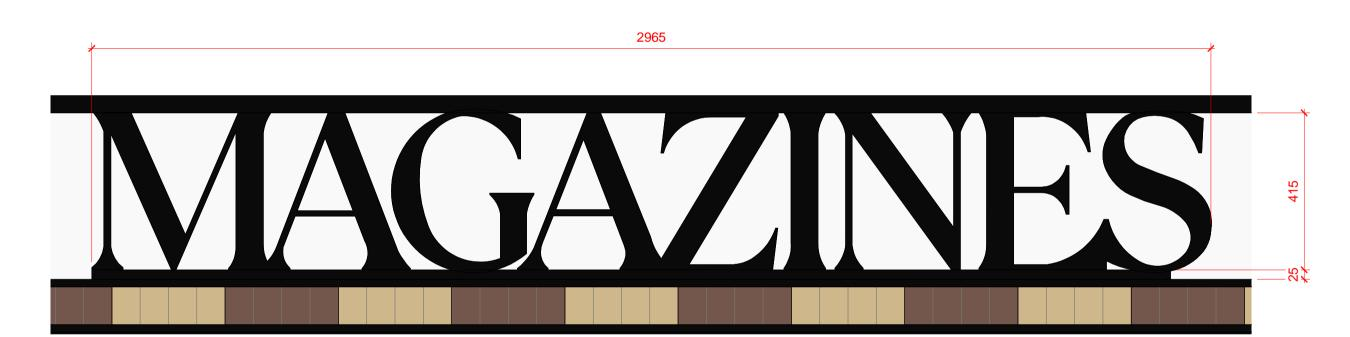
HALO ILLUMINATED SIGNAGE LED ILLUMINATION AT 4000K BEHIND OPAL ACRYLIC LETTER BACKINGS WITH BLACK LETTER FACES AND RETURNS. MOUNTED TO I BEAM DETAIL AS SHOWN ON ELEVATION DETAIL DRAWING. TOP RUNNER BAR IS NOT HALO ILLUMINATED
