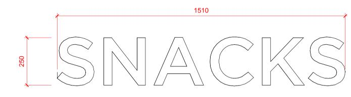
FACE ILLUMINATED SIGNAGE LED ILLUMINATION AT 4000K THROUGH OPAL ACRYLIC FACES WITH BLACK RETURNS MOUNTED INDIVIDUALLY TO BULKHEAD THROUGH FINISH.
