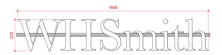
FACE ILLUMINATED SIGNAGE LED ILLUMINATION AT 4000K THROUGH OPAL ACRYLIC FACES WITH STAINLESS STEEL RETURNS MOUNTED ONTO STAINLESS STEEL CENTRAL BAR IN LINE WITH TFL GUIDELINES.
