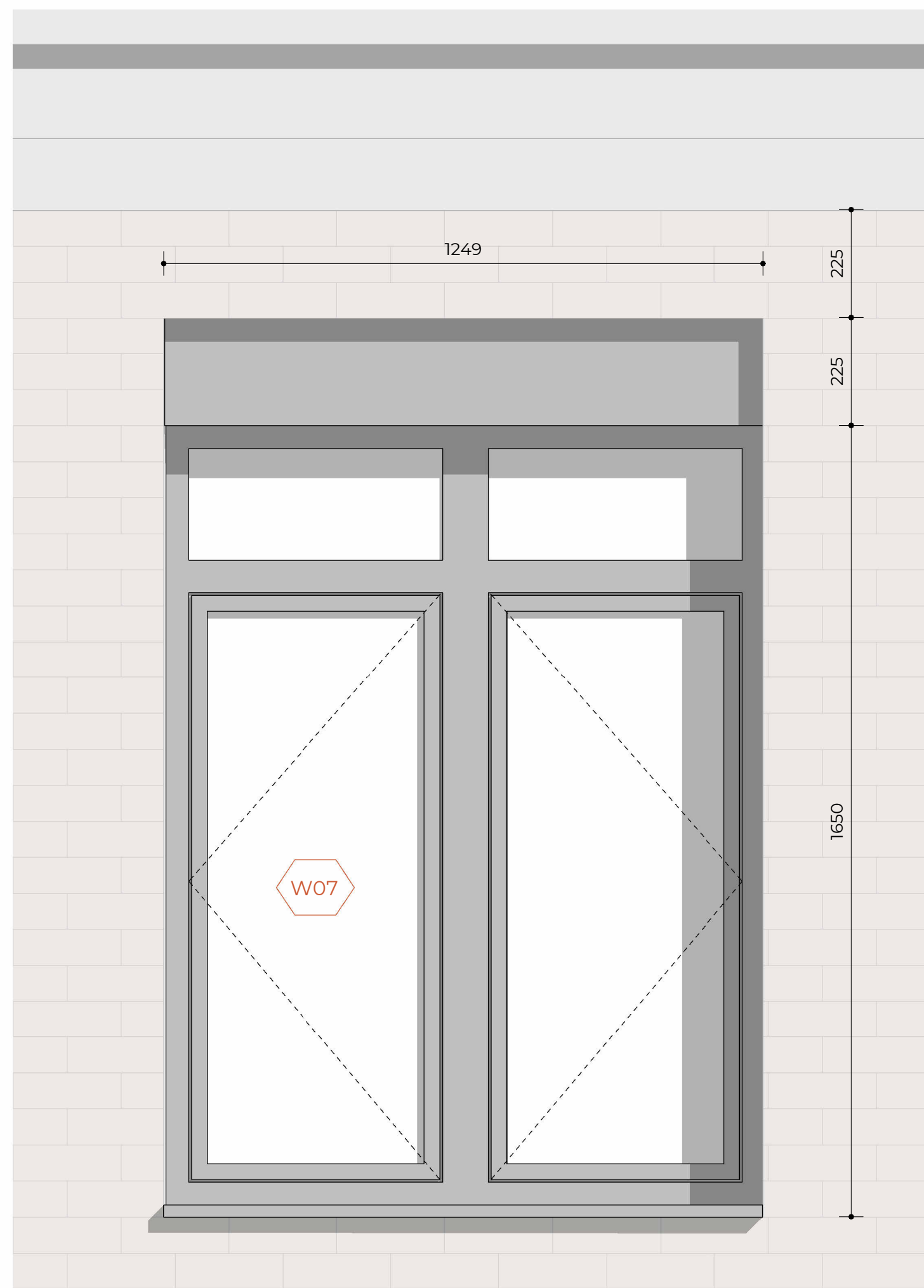
W07 - Front Elevation Third Floor
