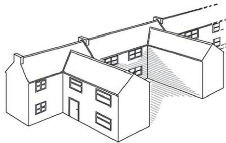
Figure 19: A tunnel effect can occur if a window is obstructed by extensions on both sides
