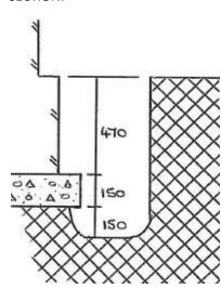
Made Ground (dark brown clayey sand with rootlets, gravel and occasional ash and brick fragments)
