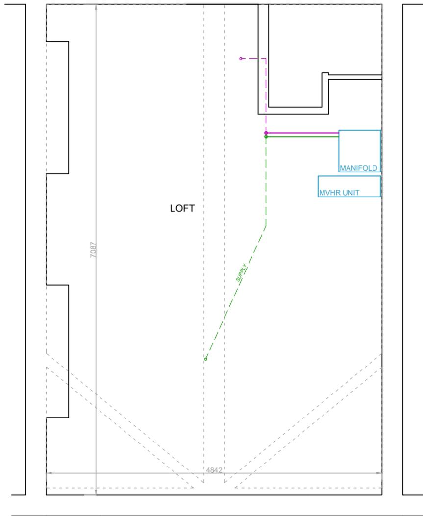
All extract and supply through 70mm ribbed ducting that does not cut through or maim any of the joists.
