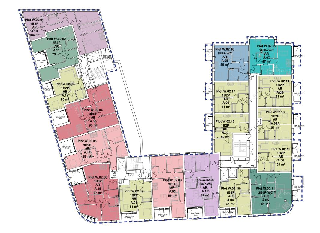
**Proposed Second Floor Plan - scale 1:250**
