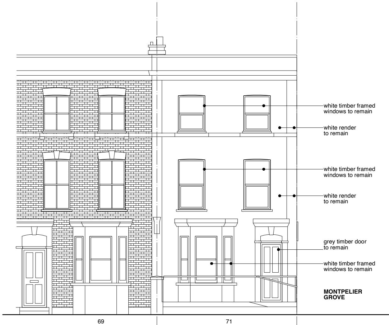
PROPOSED FRONT ELEVATION (to remain as existing)
