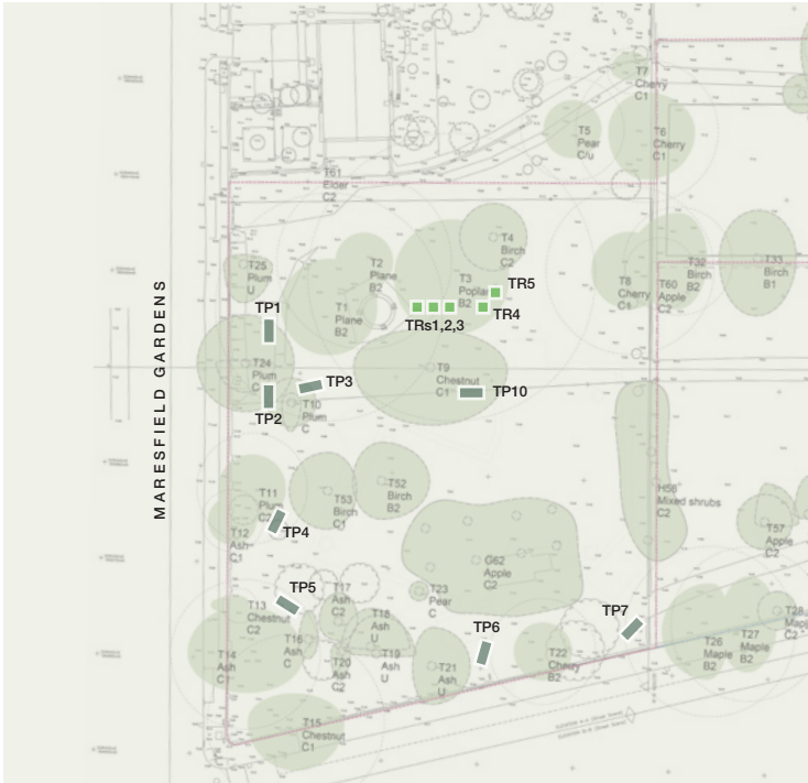
Diagram of trial pit (TP) locations, and additional trenches (TR) around the Poplar
