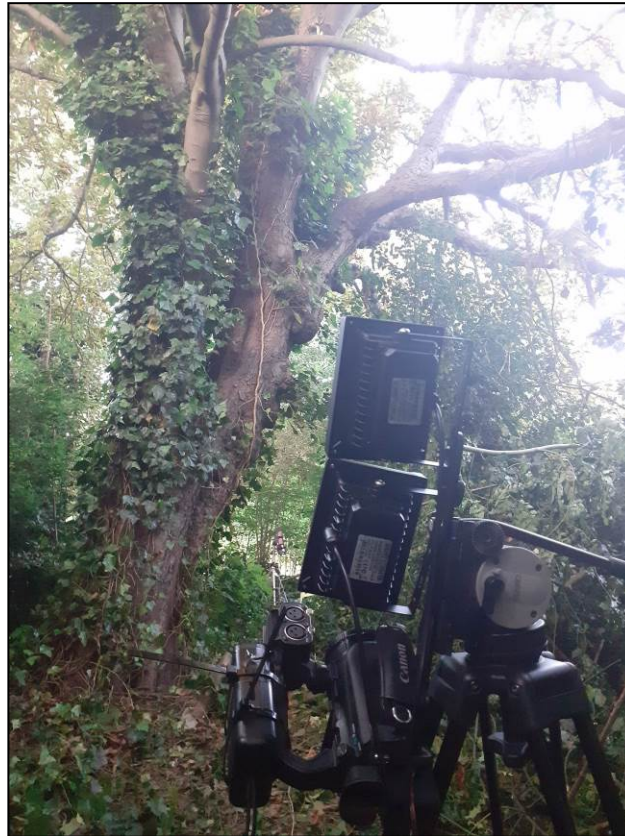
Fig 7 Survey station at the west side of chestnut (T9). The XA10 camera and IR lights, are mounted on the tripod. The Batbox Duet is mounted on the handle of the camera
