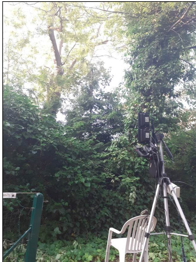
Fig 6 Survey station at ash (T42). The XA11 camera, IR lights, Peersonic (& external speaker) are mounted on the tripod. The Anabat Express detector is mounted on the chair
