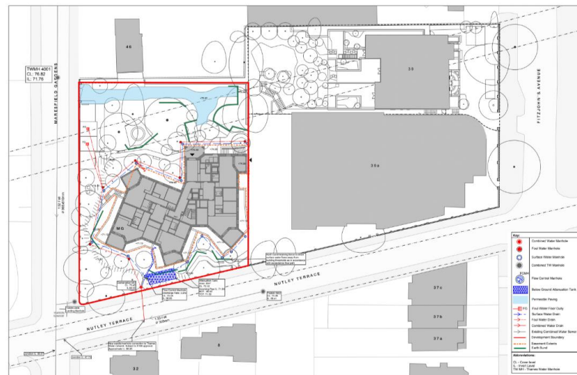
Figure 11 Maresfield Gardens drainage strategy drawing - refer to Price & Myers' drawings
