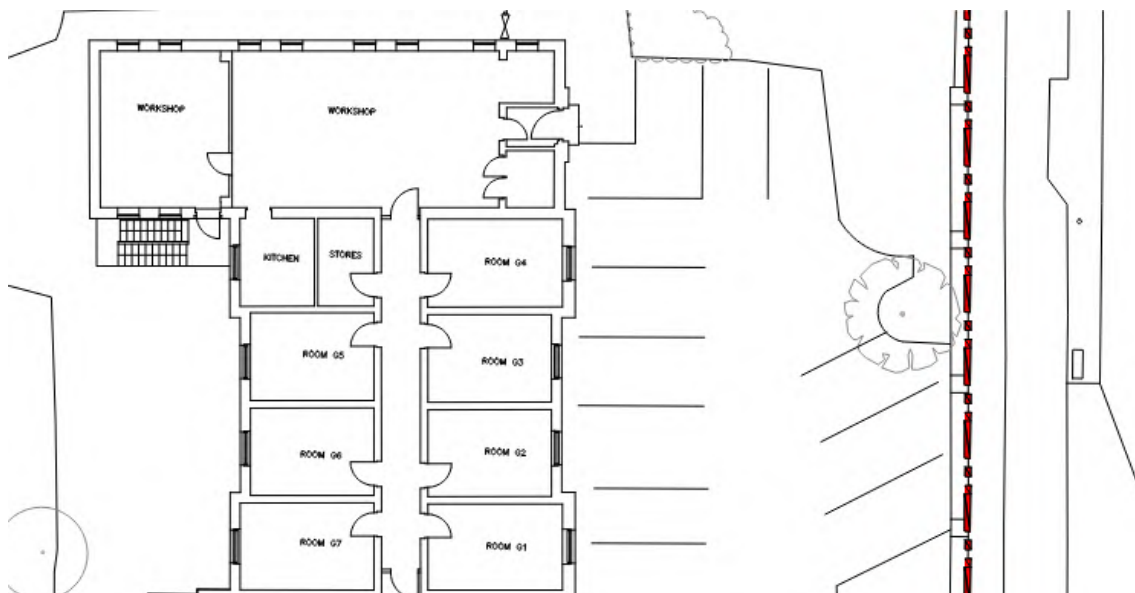
Figure 4 Ground Floor plan of the existing building
