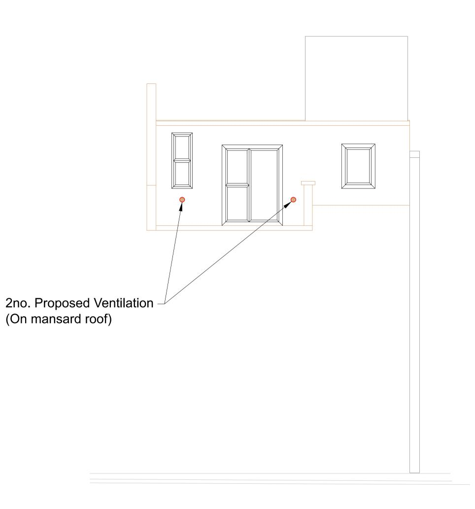
a. Location plan: 1CP01-MDS-GL-DLO-SS08\_SL23-000104 b. Existing elevation: 1CP01-MDS-GL-DEL-SS08\_SL23-000204 2. Manufacturer's recommendation is minimum 315mm to centre of core hole from internal floor level. The exact position will differ based on existing levels and internal layout/fixtures. Core holes will be aligned horizontally as best as
