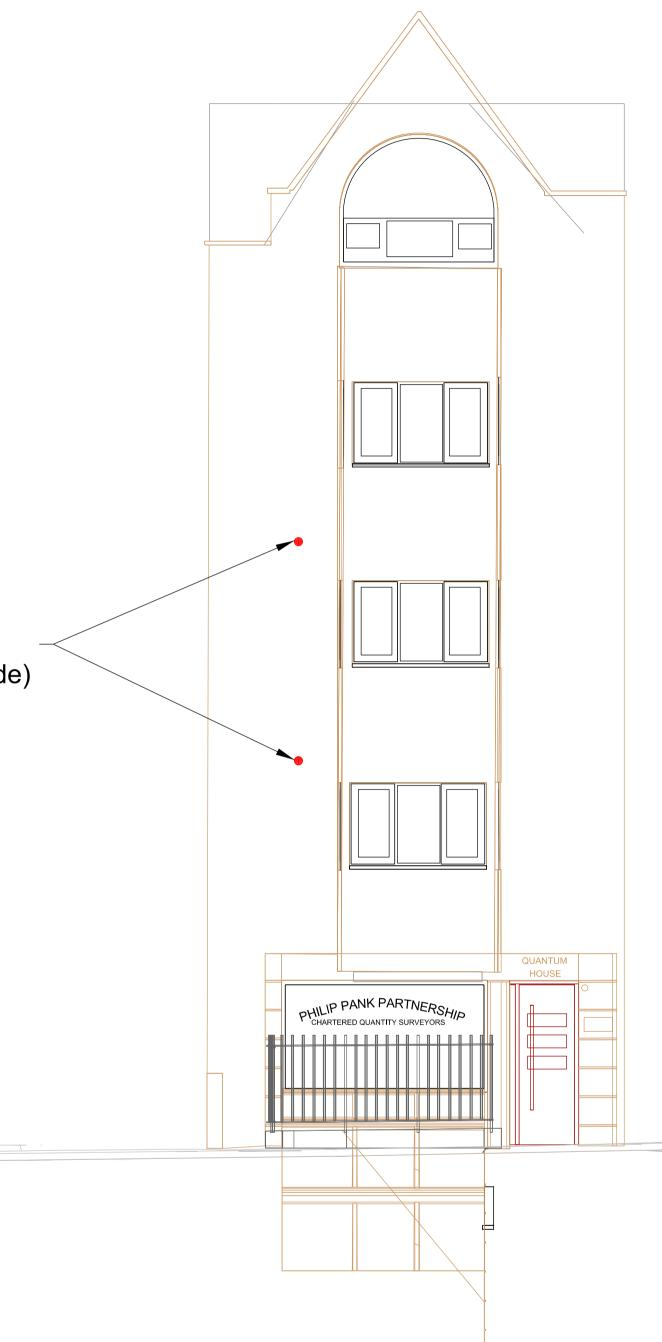
conjunction with location plan and existing elevation drawings: lan: 1CP01-MDS-GL-DLO-SS08\_SL23-000100 evation: 1CP01-MDS-GL-DEL-SS08\_SL23-000200 r's recommendation is minimum 315mm to centre of core hole floor level. The exact position will differ based on existing levels ayout/fixtures. Core holes will be aligned horizontally as best as ject to internal fixtures.
