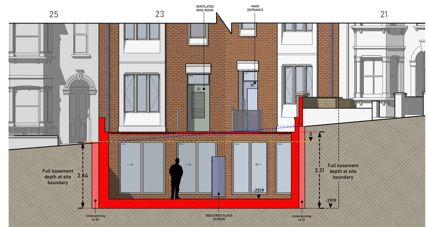
SECTION THROUGH FRONT BASEMENT LIGHTWELL
