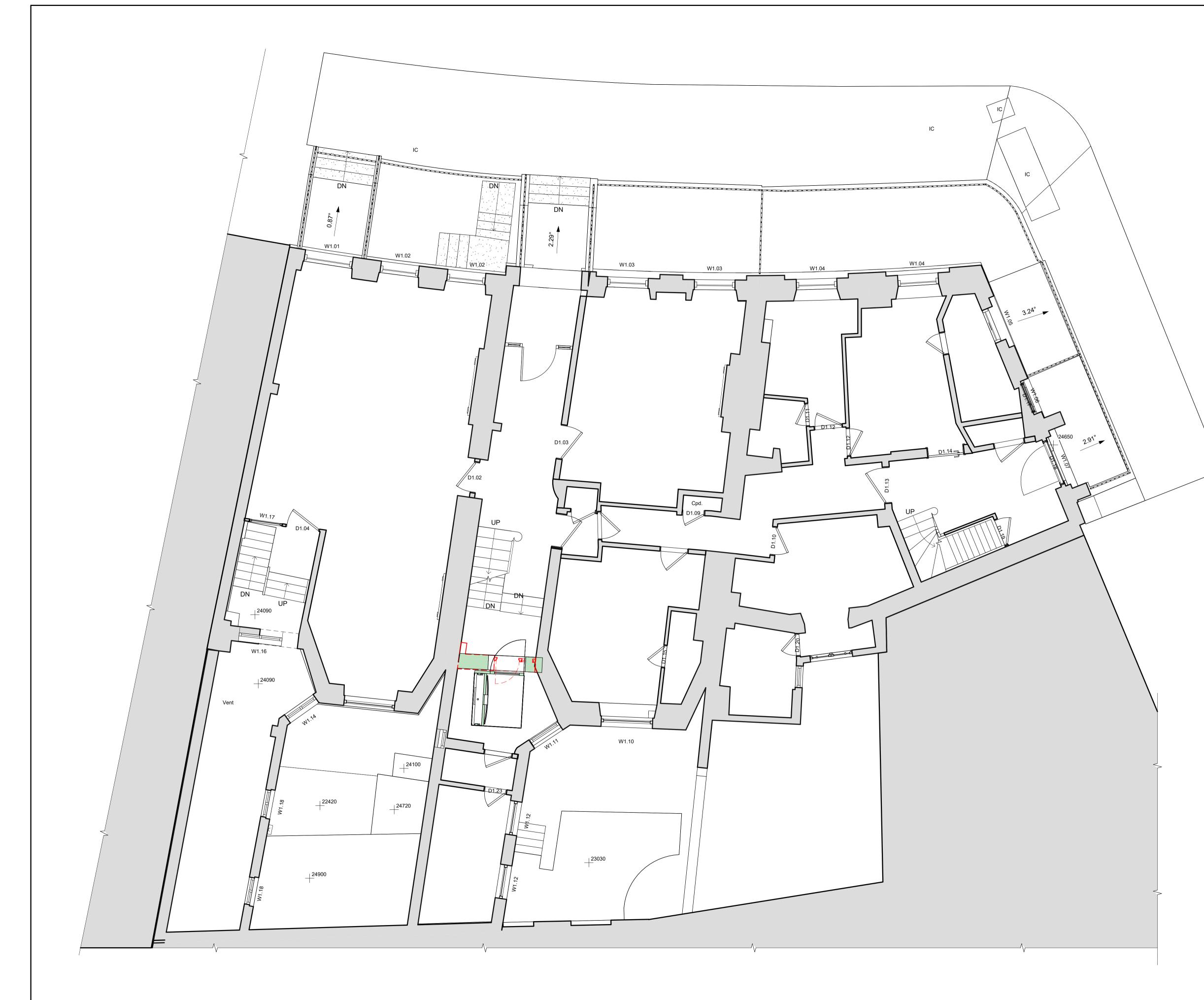
1 Proposed Ground Floor Demolition Plan 1:50
